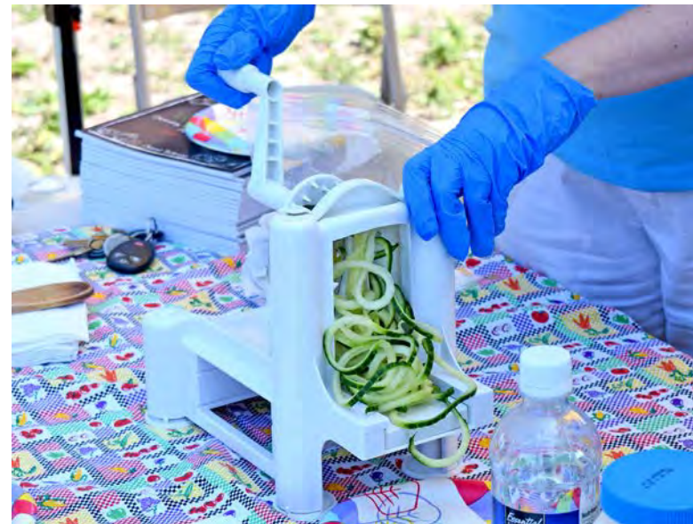
Sault Tribe Community Health registered dietitians Mary Bunker and Stacy Storey demonstrate a spiralizer, a type of inexpensive cutting mechanism used to prepare vegetables as noodles and other forms that can be used as more healthful substitutes for pasta and other foods. A close up of the spiralizer is shown here while in use during a demonstration with a cucumber. Bunker and Storey also provided folks with easily prepared samples of finished dishes prepared with the help of the spiralizer.
