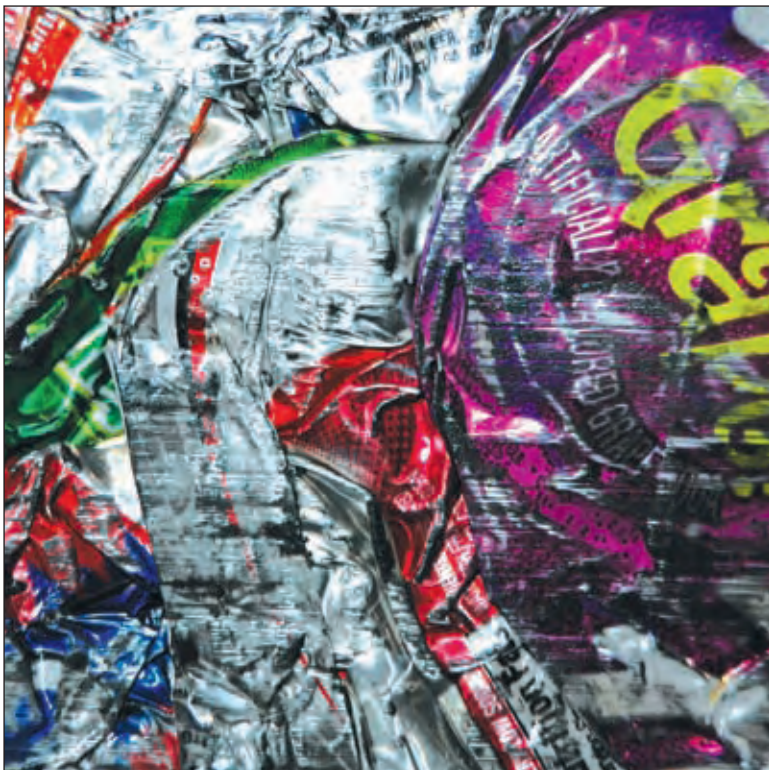
Crushed aluminum cans that have gone through the can densifier which turns them into bricks for shipping.
