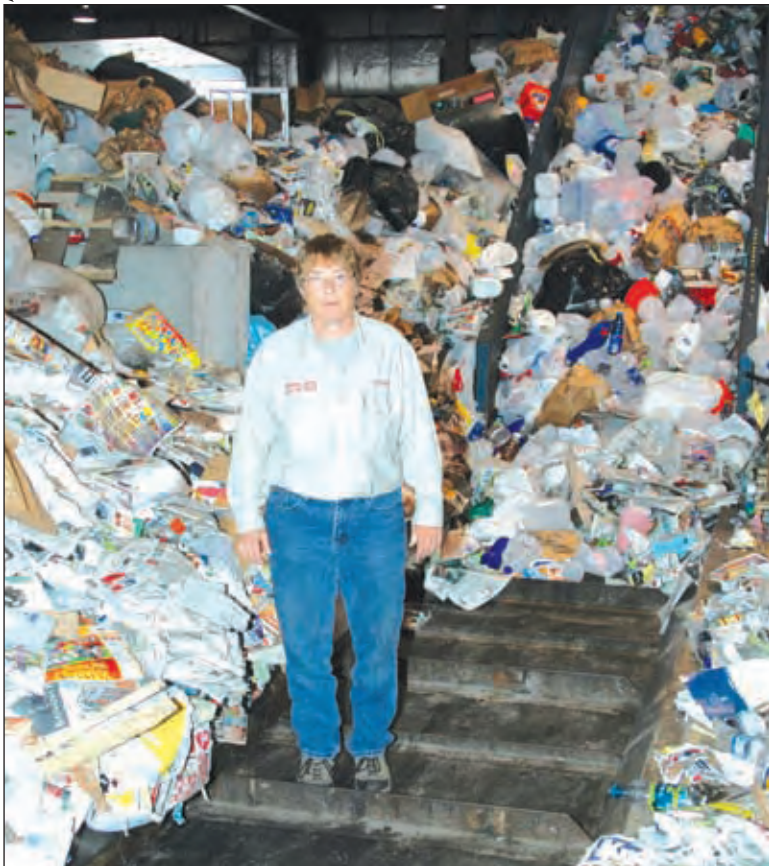
Kathy Bensel, Chippewa County Recycling Center shop supervisor, is shown here standing on the bottom of a conveyor belt which takes the product to the upper level of the building where it is sorted onto another conveyor belt for processing and bundling.
