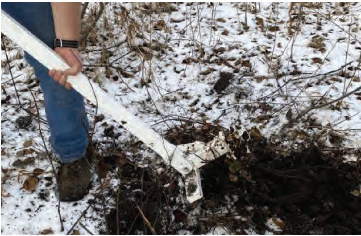
The Uprooter tool in action, a clamp is tightened around the stump and the handle is used to pull the roots out of the ground.
